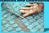
Once the carpet is cleaned and dried, the piles of the fabric are cut to level the overall height by the process of shearing. This followed by the process of embossing, in which the piles of the border of the motif are cut lower than the body of the motif. It is followed to give a good look to the carpet, as the motif seems to be protruding out of the background.
