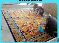
Singeing is the process of burning protruding fibers. And this done on the back side of the carpet to give it a sharp and neat finish.
