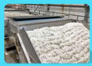
The raw wool fiber also contains lot of dust, dirt and sticky oily material called Suint. It is a wax-like material which removed by washing the fiber with caustic. Scouring completely cleans the fibers and making the fibers appropriate for further yarn processing.
