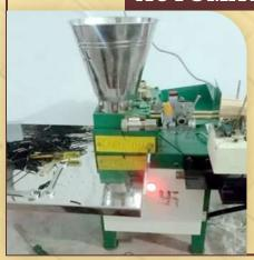
Automatic stick making machine operator is the one who produces bamboo stick using different machines such as cross cutting machine, Radial spiltting machine and stick making machine followed by polishing, bundling & Packaging.
